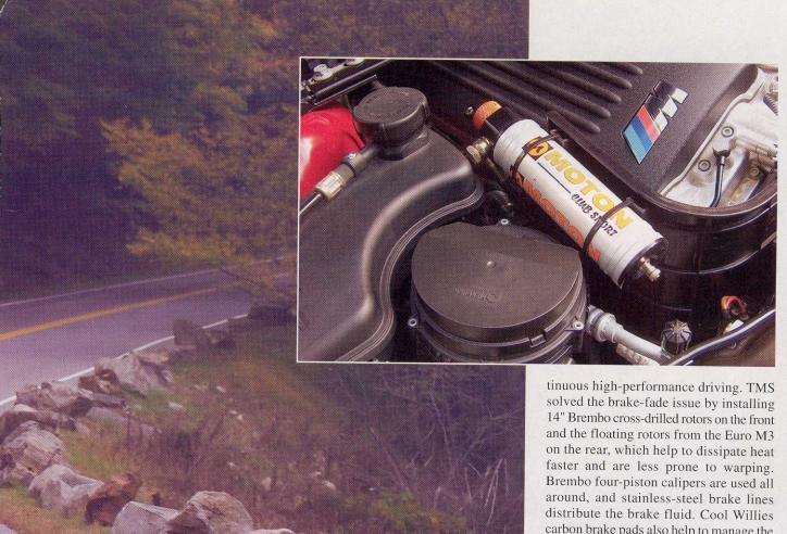
Moton double-adjustable shock absorbers have six settings for rebound and compression, providing great flexibility for street and track use.
