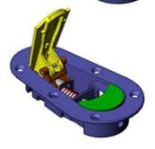
Lift Handle (retracting shear pinout of strike, releasing panel from structure)
