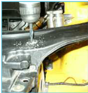
Prepare stud fixing holes. Aim to have stud at 90° to housing (±5° tolerance allows for misalignment).
