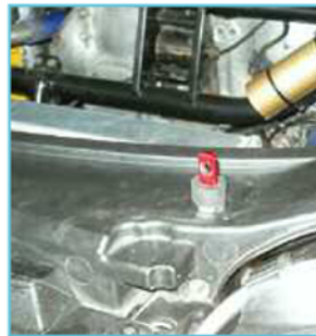
Attach stud and bump stops. Note: stud and AeroCatch axis must be at right angles to ensure smooth operation.
