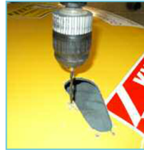
Mark and drill out fixing holes. Use AeroCatch as template (or supplied drawings – stud strike as datum point).
