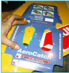
Use the template cross-hairs (narrow end to front of car) to determine AeroCatch and stud strike positions.
