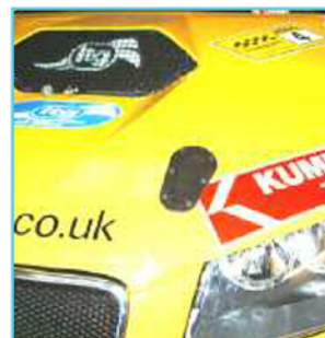
Fix AeroCatch into position. Any small radius on the bonnet may be fared round with silicone.
