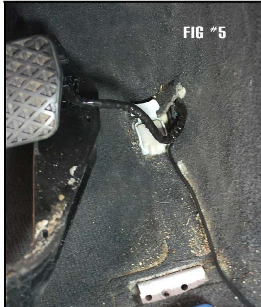
Due to lack of room beside the pedal, you will need to submerge the Sprint Booster into the carpet to allow reinstallation of the pedal. The slit made earlier makes this possible. Shown in Fig #5
