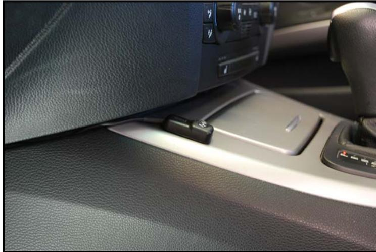
**You have now completed the Sprint Booster installation. From here you can alter the degree of response in the pedal by pressing the button on the lead installed on the center console. Red denotes the most responsive setting, green slightly less and no color in the button returns the car back to stock.**
