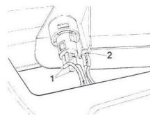
Remove the cigarette lighter and ashtray. The ashtray is held in place with 2 screws on the backside of it. Unscrew them and pull up on the ashtray. Disconnect the wires from the cigarette lighter and ashtray light. Set them aside.
