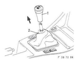
Next remove the gear lever. This is accomplished by putting the car into second (2<sup>nd</sup>) gear and pulling up hard on the shift knob itself. Pull on the knob - not the boot underneath it. Next pull the boot from the center console. The boot is held in place by plastic clips. You can feel where the clips are and are not by tugging along the edges.
