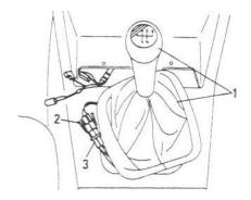
Run the supplied shifter wiring harness through the opening in the gear lever boot. Place the Illuminated Shift Knob and boot over the shift lever but do not secure them in place. Connect the car's cable to the shifter's harness.
