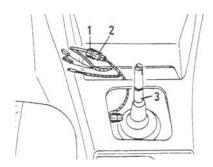
Connect the car's plug from the dash onto the new plug. Run the other end of the wire to the gear lever by going under the center console.
