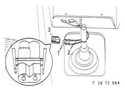
Push the cable plugs onto the end of the exposed wires and crimp them firmly down (#'s 1 & 2). Click the cable plugs into the plug (#3 in the picture to the left). The plug is marked "1" and "2". The brown/green wire corresponds to hole 1. The green/red wire goes to 2. They will snap into place with an audible "click" and should not come loose.
