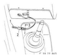
Pull the bulb (#1) from the end of the wire on the lighter's cable (#2). Now cut the wires as shown at #3 in the picture to the left. Remove about 1/8" of the insulation from the wiring.
