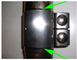
**15.** Lift the mid-section with Test Pipes into vehicle. Loosely install hardware for the transmission tunnel cross brace, rear clamps, and front flange bolts and nuts. Check alignment the of the full exhaust system and tighten all hardware including all exhaust clamps at this point. Recheck alignment of full exhaust system.
