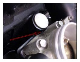
3. Ensure the throttle body has its profile gasket installed (source a new one if it does not). Bolt throttle body onto adapter plate with 6mm bolts Note: there are six tapped hole in the adapter plate use the holes show in center image.
