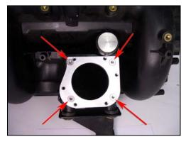
2. You will need to remove some material from the throttle body to clear the idle control valve port on the intake manifold. Remove approximately 4mm deep and 28mm high of material from throttle body bolt boss. Note be careful not to damage electronics with heat or vibrations when removing material.
