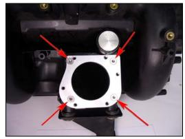
2. Place a ring of sealant on the throttle body mounting surface. Bolt throttle body onto adapter plate with 6mm bolts Note: there are six tapped hole in the adapter plate use the holes show in center image.
