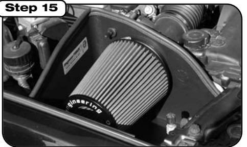
Make sure all hoses and clamps are tight and that all electrical components (if applicable) are secure. Check and retighten connections and filter after a few hours of operation.
