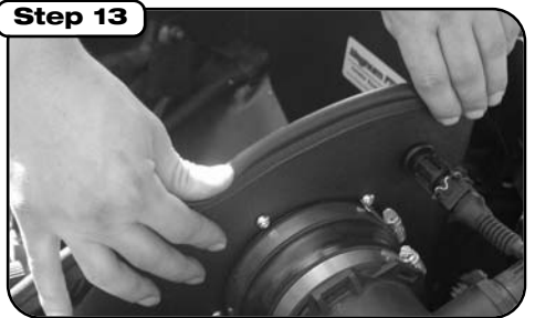
Install trim seal.
