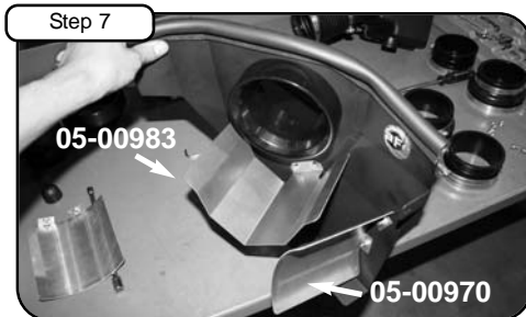
Step 7 Attach air diverters to housing using button head and wavy washers. Tighten using 5mm allen key. Install 3/4" trim seal on housing. Note: Failure to install air diverters may result in CEL (Check Engine Light).
