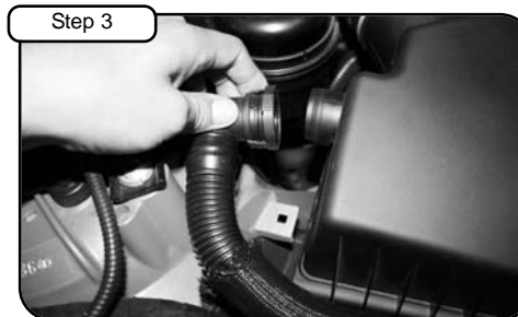
Step 3 Disconnect smog line from air box.
