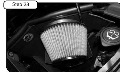
Step 28 Install air filter and tighten using 5/16" nut driver. Install pre filter. Make sure cap is installed in filter top. Re-connect MAF sensor harness.
