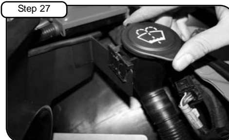
Step 27 Place washer inlet reservoir onto housing tab.
