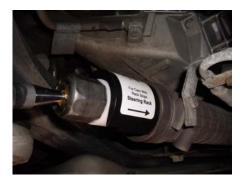
If your car does not have Rack Stops, locate the side of the tool that reads: "For Cars Without Rack Stops" The arrow corresponds with this application only. Arrow points to center of car when installed.
