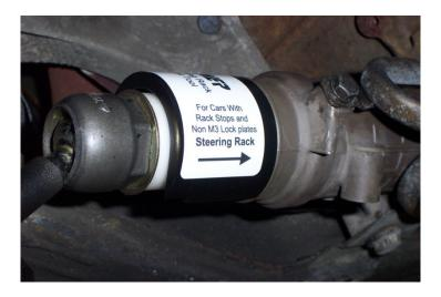
If your car has an M3 lock plate but without Rack Stops, locate the side of the tool that reads: "For cars With M3 Lock Plate but without Rack stops" The arrow corresponds with this application only. Arrow points to center of car when installed.
