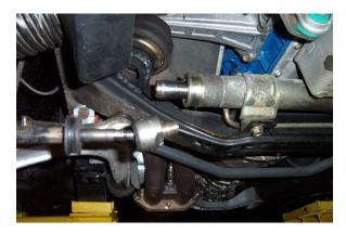
5. Take the appropriately colored rack stop, and evenly push it on the shaft until it is flush with the end of the shaft. The use of a block of wood and a hammer to evenly tap it on may be required.
