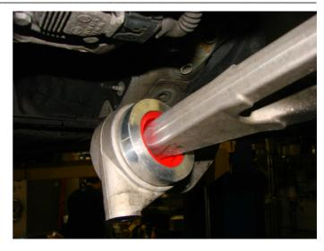
Step 8. Reattach factory lollipops to chassis. Reinstall factory reinforcement plate. Test drive.
