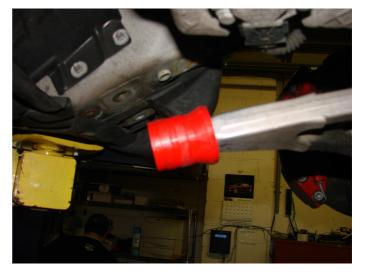
**Step 6.** Lubricate the outside of the urethane bushing as well as the inside of the FCAB housing. Start to push (and twist) the FCAB housing assembly onto the urethane bushing. You can use the deadblow hammer to get it started.
