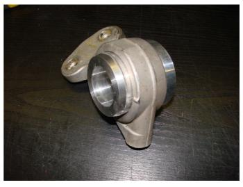
**Step 5.** Spray some windex on end of the control arm and inside the supplied urethane bushing. Using a deadblow hammer, pound bushing onto end of control arm until flush.
