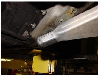
**Step 4.** Push out the factory bushing from the factory FCAB mount. Note that the E46 M3 lollipops have a small "bump". It is VERY important that the TMS FCAB housing is pressed in from the OTHER side of this bump.
