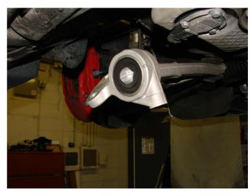
**Step 2.** Using a bushing removal tool, remove the factory lollipop and bushing from the factory control arm.
