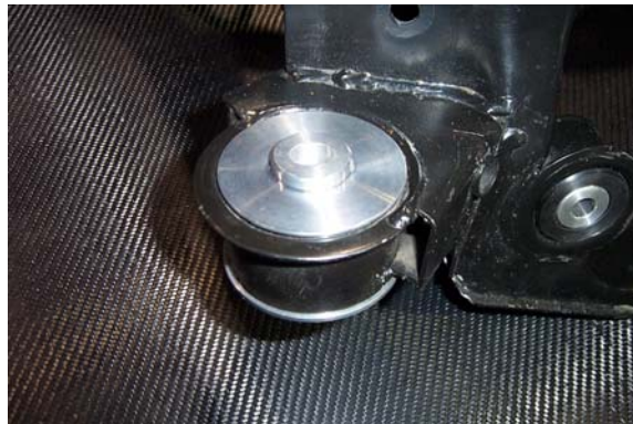
Figure 3: Finished front bushing- sleeve with radius and slot is installed on top of sub-frame. Sleeve with no radius and slot is installed on bottom of subframe.
