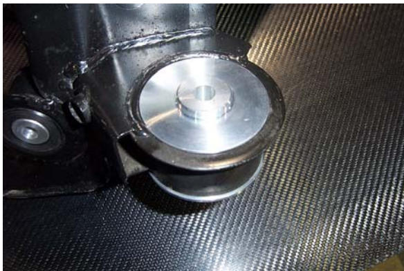
Figure 2: Finished front bushing- Sleeve with radius and no slot is installed on top of sub-frame. Sleeve with no radius or slot is installed on bottom of sub-frame
