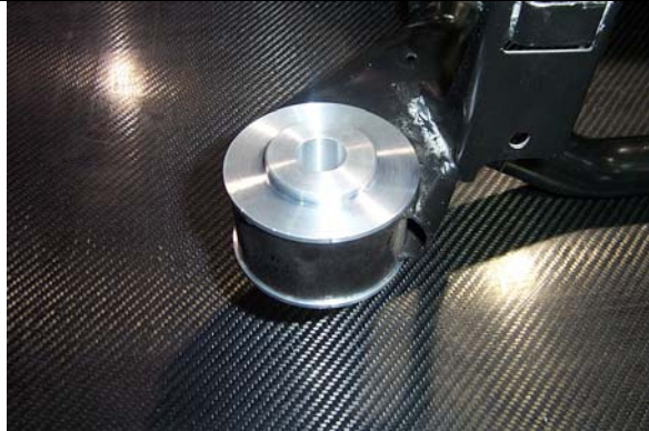
Figure 1: Finished Rear bushing- Sleeve with shortest length is installed on bottom of sub-frame. Sleeve with longest length is installed on bottom of sub-frame
