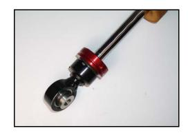
13. Slide the shock and bushings assembly into shock mount by raising the lowering control arm up while making sure the spring is seated. Install shoulder bolt through the mount and shock bearing and install 8mm washer and nut. Torque to 18 ft. lbs.
