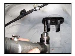
11. Insert small bolt and washer from the inside of the car. Then, apply the washer and nut onto bolt from the underside of the vehicle. Torque the 16mm bolt from the inside of the car to 100 Ft. Lbs. check the tightness of the 4mm nut and bolt. (As you torque the 16mm bolt, pressures on the 4mm nut and bolt are being relieved.)
