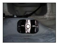
10. Using a 5/32" or 4 mm drill bit, drill one hole through the chassis, using the mount as a template. Note each mount just needs one 4 mm bolt. It is to keep the mount from spinning when tightening the 16mm bolt. We suggest using the hole closest to the rear of the car.
