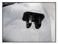
8. Install cap with bolt and washer from inside the trunk. Bolt should be tightened so it is slightly snug.
