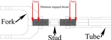
**Please note on the diagrams below:** after the camber arms are fully installed and the Jam-Nuts have been tightened, your threads should match the diagram on the left. The diagram on the right shows an incorrect assembly.
