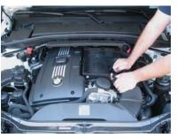
Unclip the wire harness above the air filter box
