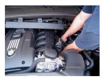
Slide a guitar pick between the lock and catch to loosen the TMAP connector
