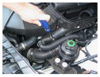
Squeeze and unclip the vacuum connection and unhook vacuum line
