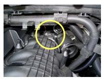
The TMAP sensor circled in yellow is on the intake tube before the throttle, the connector is facing down
