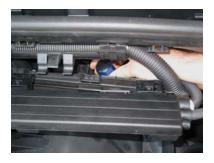
The airbox is held by three rubber mounts, the front one is circled in vellow
