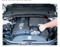
Slide off the inlet from the front of the airbox
