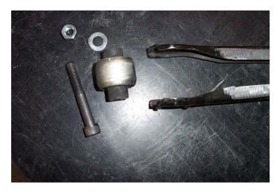
3. Align the reinforcement to evenly cover the split in the camber arm. Place the reinforcement 3 ½" from the wide end of the arm.
