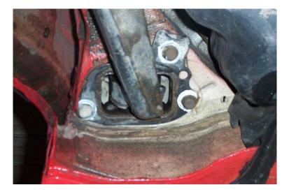
**3.** Remove brake line bracket from rear trailing arm
