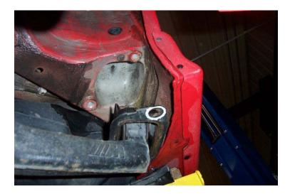
**5.** Remove the bolt through the center of the toe plate bracket.
