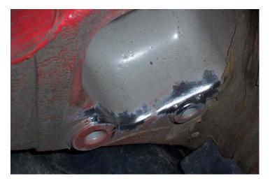
2. -Finish the weld around each of the mounting studs.
