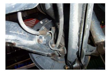
4. Remove the 3 bolts that connect the toe bracket to the chassis
