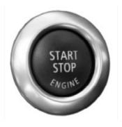
Start the engine and let it idle. As long as the car starts and idles normally you can now turn it all the way off. You can ignore any error messages in the iDrive screen (you will clear fault codes and adaptations in the next step).
