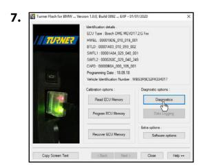
The first action is to check for existing fault codes in your ECU. This is also a communications test between your car and the Turner Flash tool.
