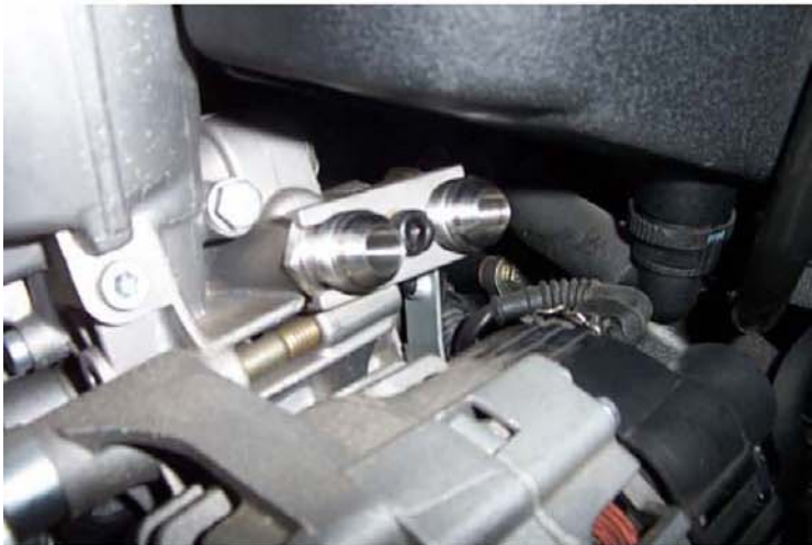
Fittings installed on housing with no hose
