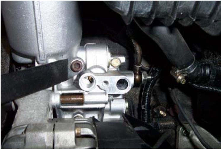
Oil Lines removed
