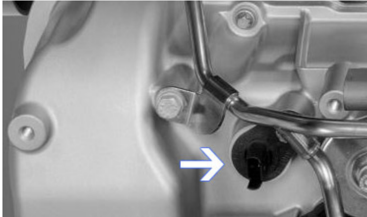
Camshaft sensor location on valve cover.
