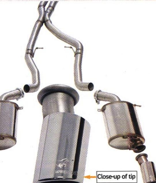
exhaust right after the stock catalytic converters
