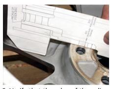
6. Verify that the edge of the caliper does not touch the rim or the wheel spokes. A minimum clearance of 2mm (0.080") is recommended.
